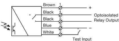
\* Relay type: Open when SGR not powered
